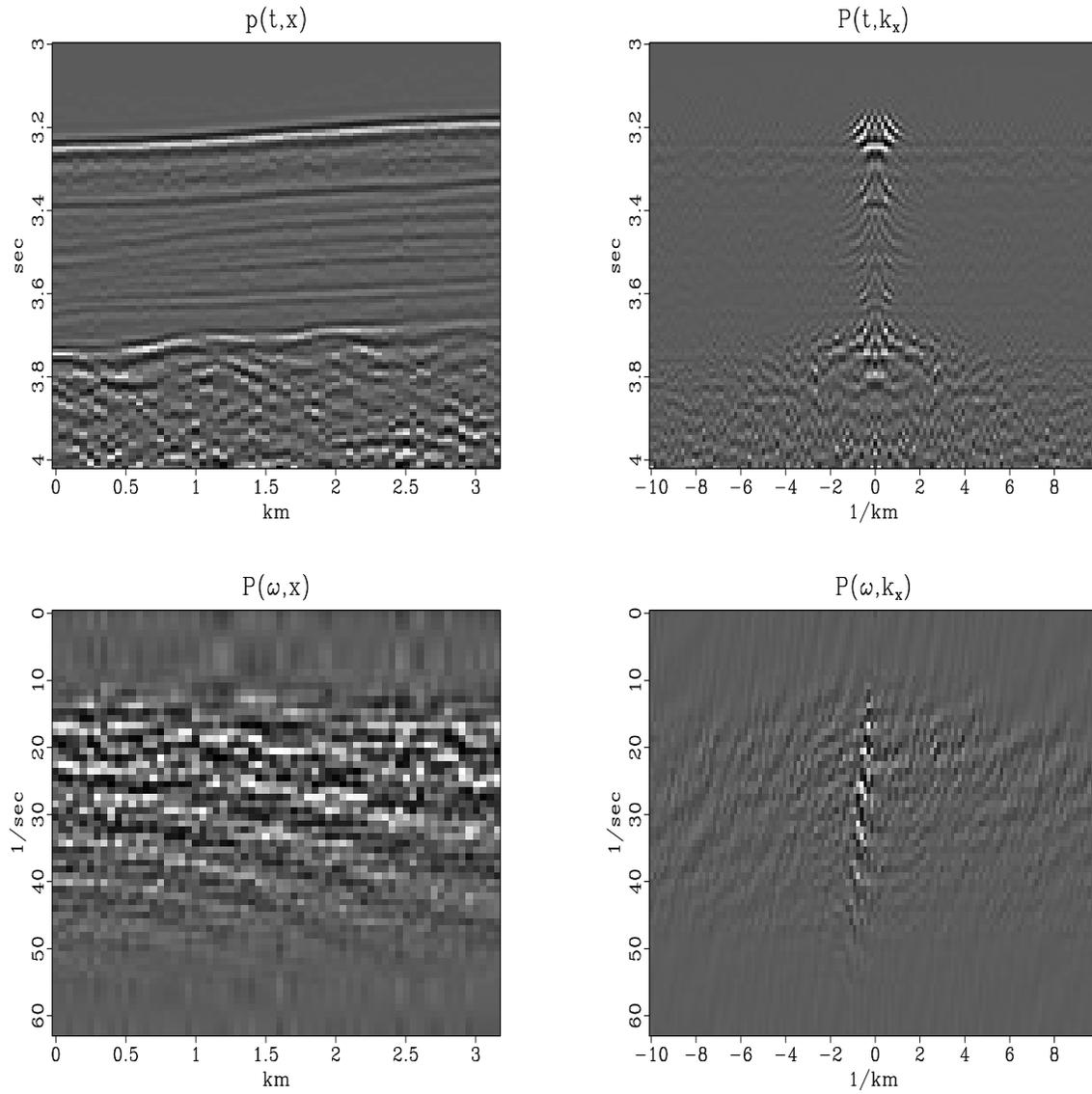
Figure 4: A deep-marine dataset  $p(t,x)$  from Alaska (U.S. Geological Survey) and the *real* part of various Fourier transforms of it. Because of the long travelttime through the water, the time axis does not begin at  $t = 0$ .
