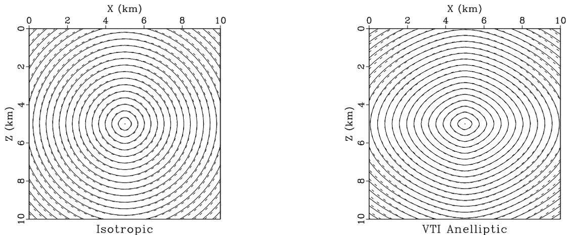
Figure 8: Finite-difference wavefronts in an isotropic (left) and an anisotropic (right) homogeneous media. The anisotropic media has the parameters of the Greenhorn shale. The finite-difference sampling is 100 m. The contour sampling is 0.1 s. Dashed curves indicate the exact solution. The finite-difference error will be reduced at finer sampling.
