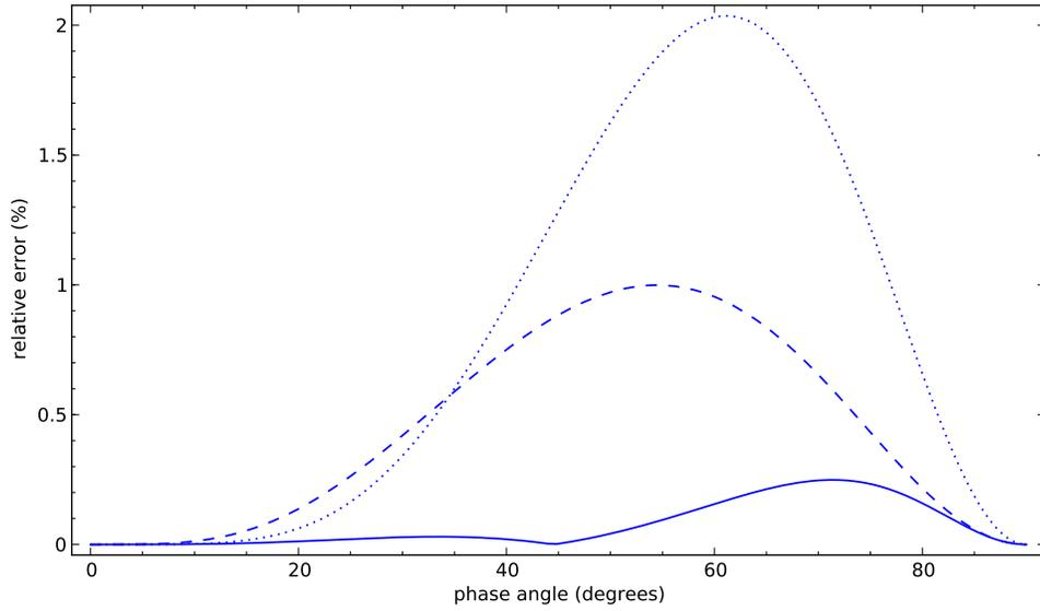
Figure 5: Relative error of different group velocity approximations for the Greenhorn shale anisotropy. Short dash: Alkhalifah-Tsvankin approximation. Long dash: Zhang-Uren approximation. Solid line: suggested approximation.
