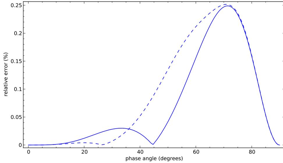
Figure 6: Relative error of different group velocity approximations for the Greenhorn shale anisotropy. Dashed line: Alkhalifah approximation. Solid line: suggested approximation.
