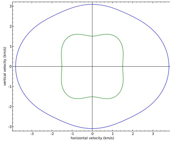
Figure 1: Phase velocity profiles for  $qP$  (outer curve) and  $qSV$  (inner curve) waves in a transversely isotropic material (Greenhorn shale).
