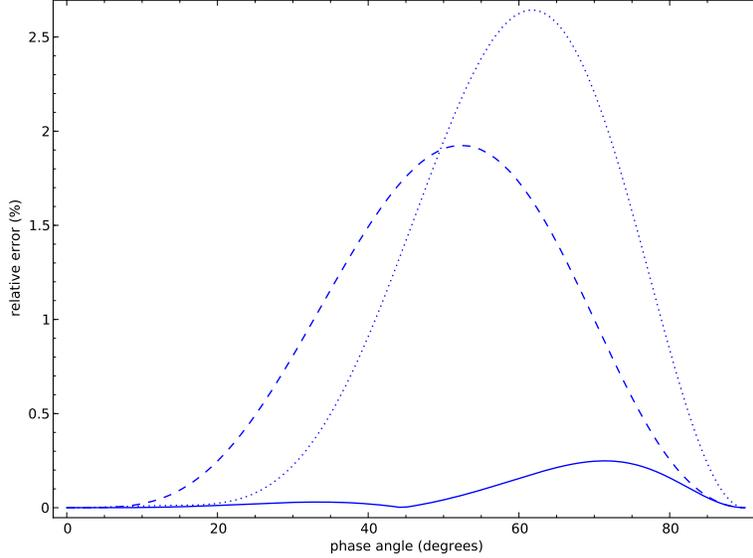
Figure 4: Relative error of different group velocity approximations for the Greenhorn shale anisotropy. Short dash: Thomsen's weak anisotropy approximation. Long dash: Muir's approximation. Solid line: suggested approximation.
