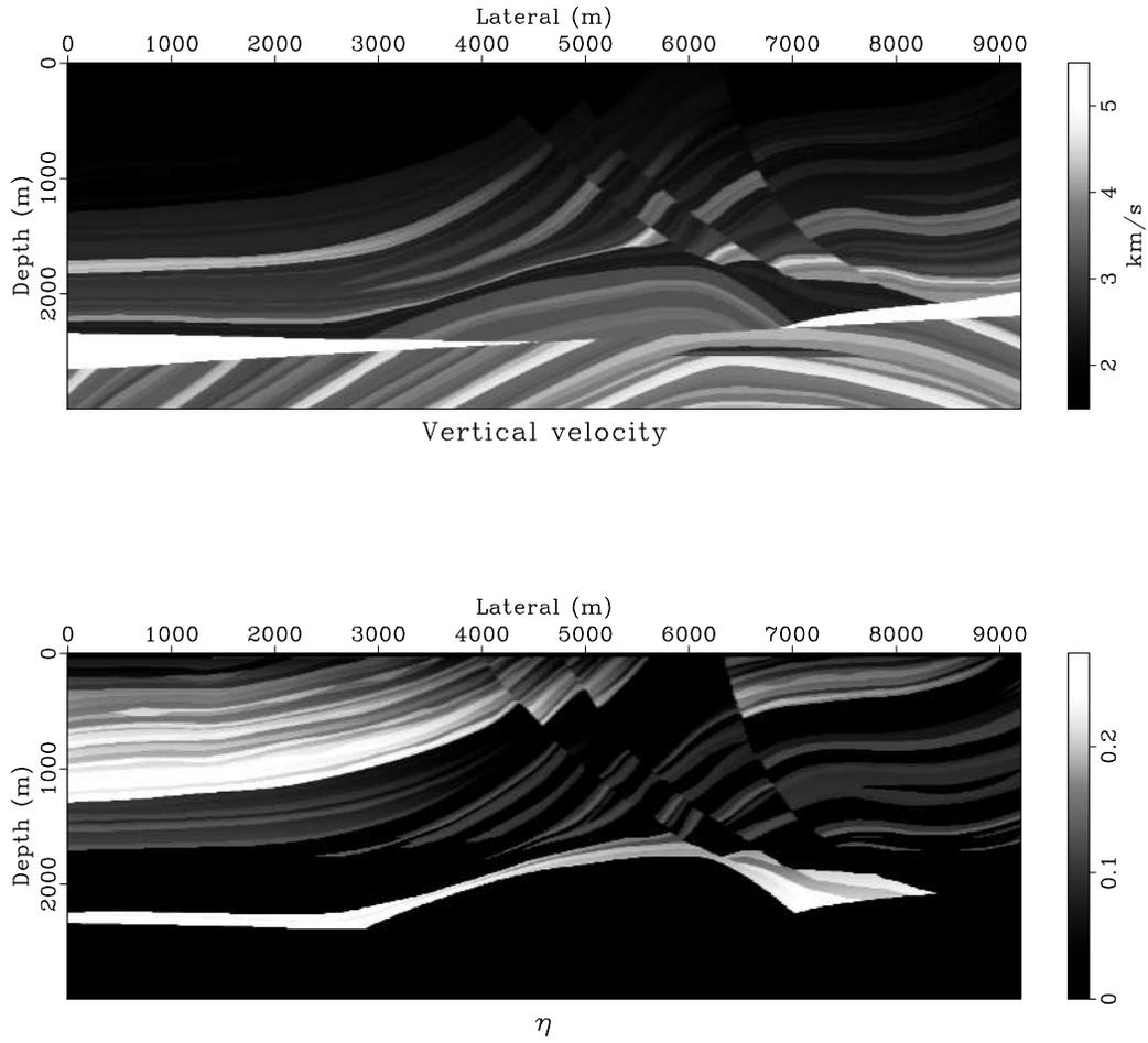
Figure 10: Alkhalifah's anisotropic Marmousi model. Top: vertical velocity. Bottom: anelliptic  $\eta$  parameter. The vertical velocity is taken equal to the NMO velocity  $V_n$ .
