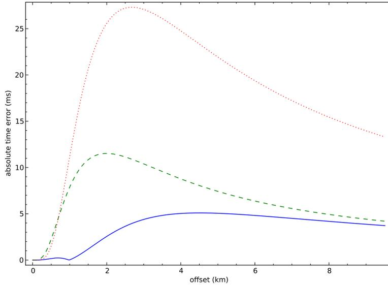
Figure 7: Traveltime moveout error of different group velocity approximations for Greenhorn shale anisotropy. The reflector depth is 1 km. Short dash: Alkhalifah-Tsvankin approximation. Long dash: Zhang-Uren approximation. Solid line: suggested approximation.
