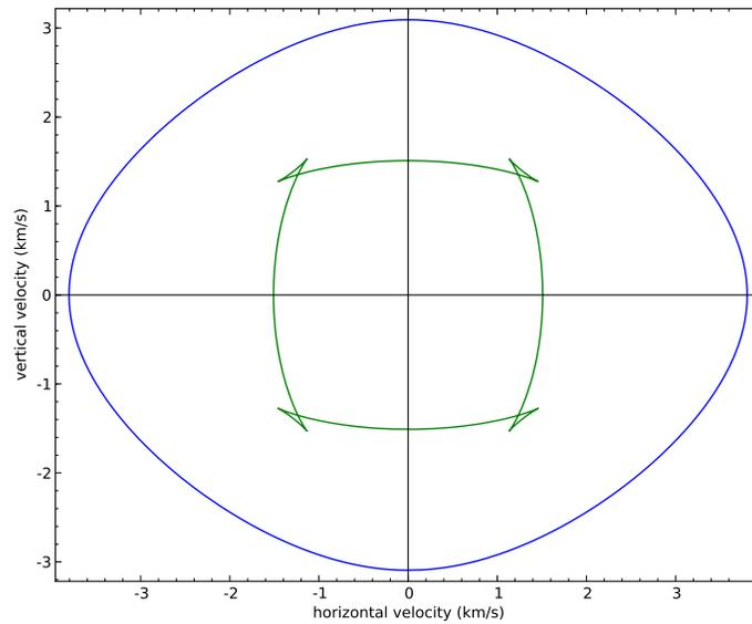
Figure 2: Group velocity profiles for  $qP$  (outer curve) and  $qSV$  (inner curve) waves in a transversely isotropic material (Greenhorn shale).
