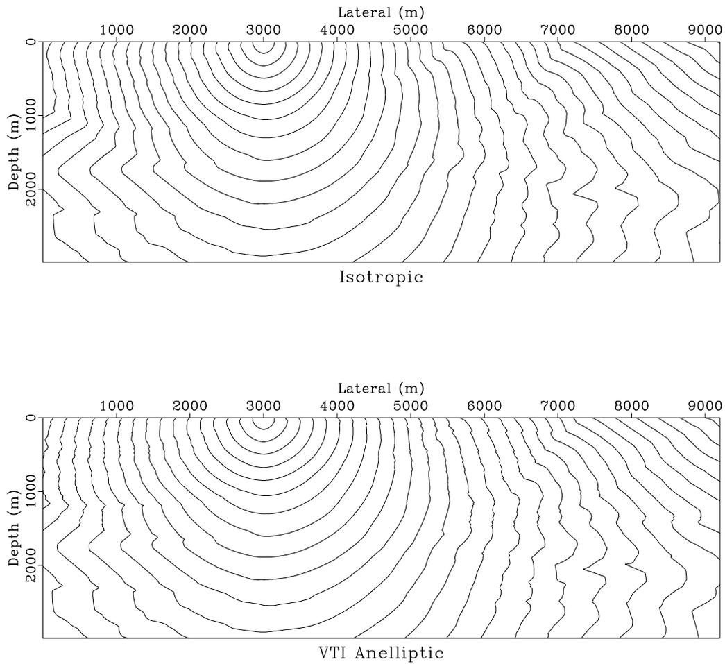
Figure 9: Finite-difference wavefronts in the isotropic (top) and anisotropic (bottom) Marmousi models. A significant shift in the wavefront position suggest possible positioning error when seismic imaging does not take anisotropy into account.
