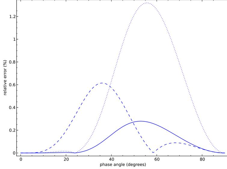
Figure 3: Relative error of different phase velocity approximations for the Greenhorn shale anisotropy. Short dash: Thomsen's weak anisotropy approximation. Long dash: Muir's approximation. Solid line: suggested approximation (similar to Alkhalifah's acoustic approximation.)
